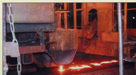
Molten iron being poured into moulds to form brake-disc castings in the foundry of Precision Disc Castings.
