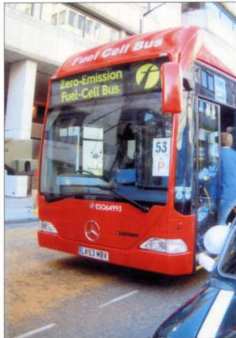
The Mercedes Citaro hydrogen-fuelled bus which participated in last year's Lord Mayor's Show
