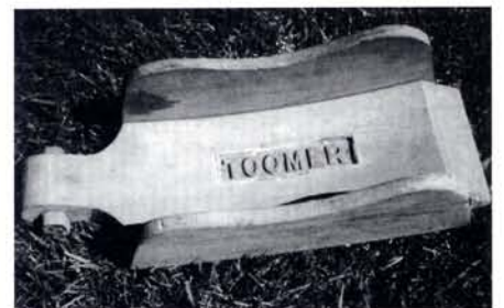
This wooden pattern was used to produce cast-iron braking shoes for Toomers, the Reading coal merchants.
